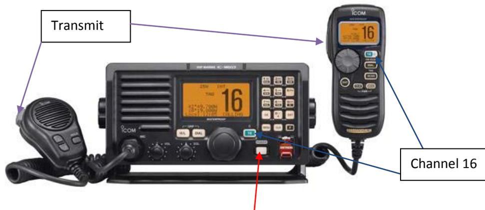
Switch on the VHF by pushing the white “Power” button on the main unit.
